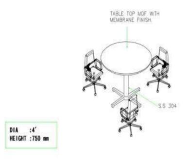
**Specifications:** Table top should be made up of MDF with membrane finish. Understructure should be made of stainless steel with grade S305.
