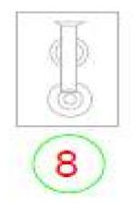
**COMBINATION:** It provides a complete safety for immediate first aid. In one location both Eye/face wash function & drench ensure instant flushing of the eyes /body with enough water. Shower and eye wash are operated simultaneously or independent either by push lever or foot operation. Recommended water pressure 30 psi 110 liters per minute.
