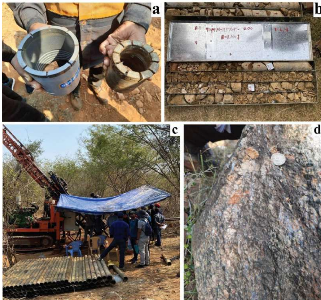
Figure 4 (a) Diamond drill bit with the casing, (b) Core Sample in a box pattern, (c) Drilling site for Molybdenum, (d) Mylonitized Epidotite Hornblende Gneiss.
