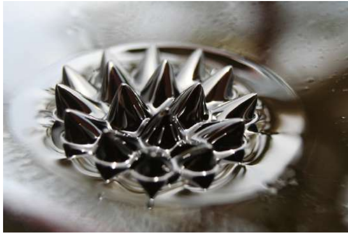
Figure 69: Ferrofluid spikes when a ferro fluid is subject to a magnetic field
