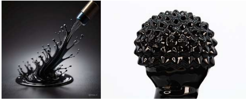
Figure 70: Spiky structures of ferro fluids
